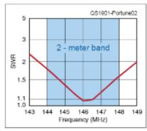
Figure 2 — SWR plot of the slot-cube antenna.
